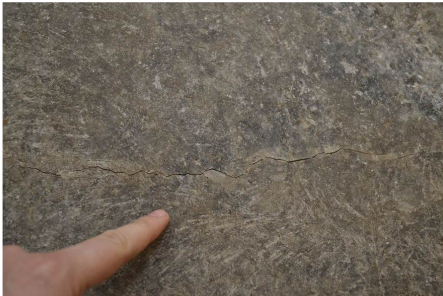
Fig. 9. Fractures occurring due to cooling
